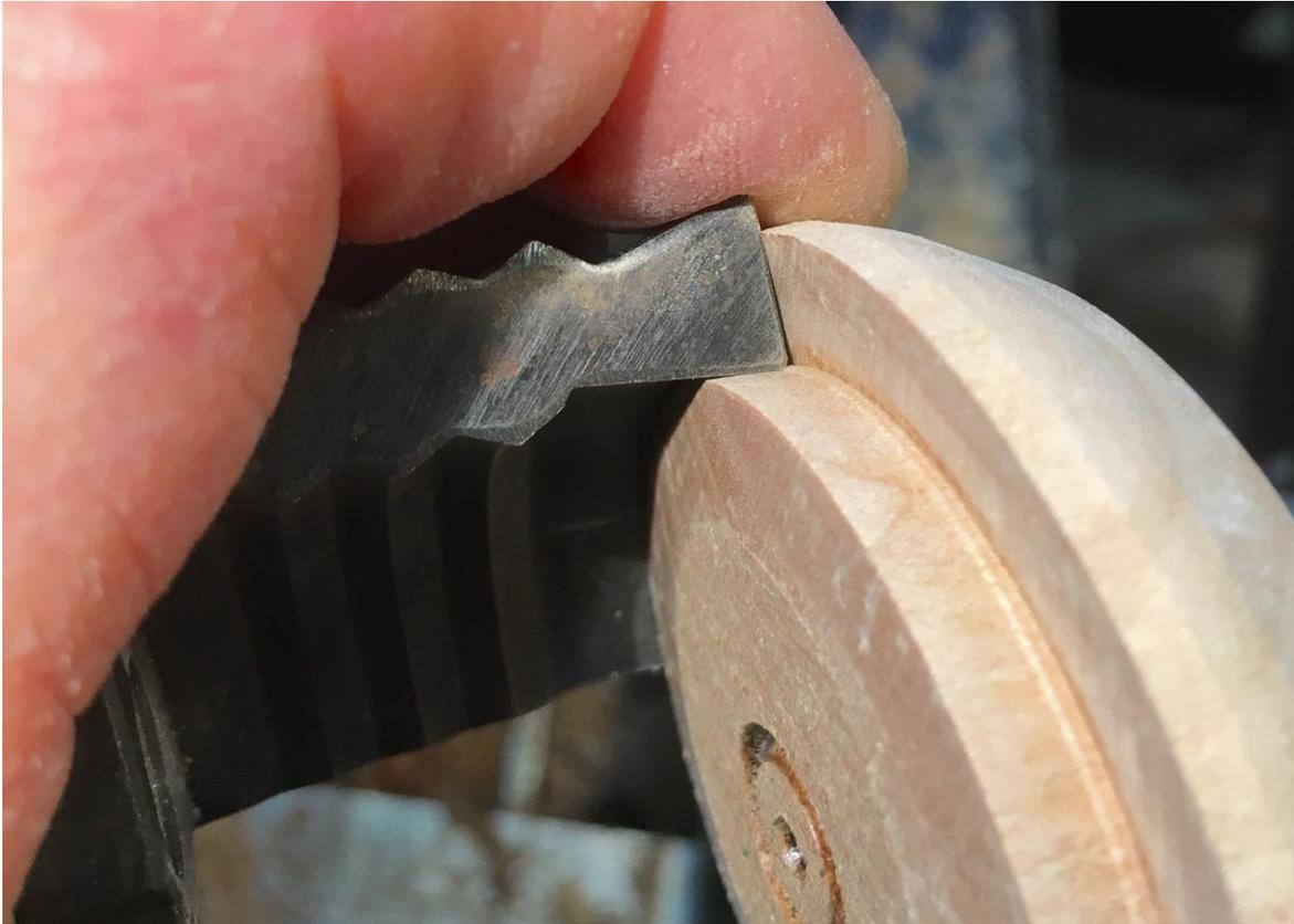
This tenon (the bowl has been finished and removed) was a very good fit for these dovetail shark jaws. When the bowl was reversed, it ran perfectly true.
