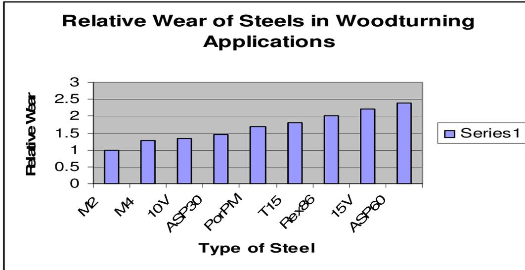
**SUMMARY OF THE RESULTS** M2 is used as the reference and is given a wear resistance of 1.0. Everything else was measured relative to that. You can see that a number of common steels are listed with ASP60 (also known as 2060) being the “best” with about 2.4 times the wear resistance of M2. These results “feel” right to me. I have M2, M4, ASP30, ProPM, and ASP60 gouges and they do perform just about how this chart predicts they should.
