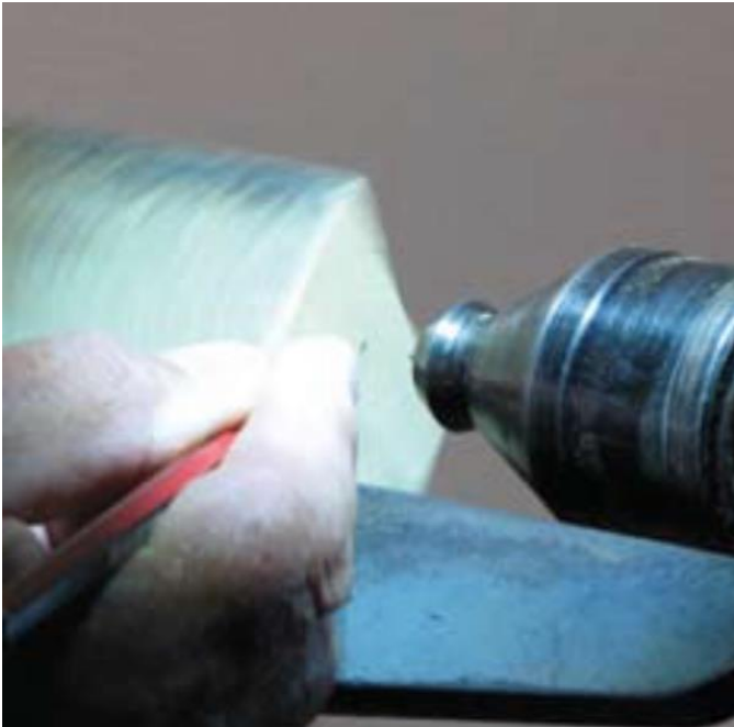
Figure 4. Marking the end of the rotating wood with a pencil.
