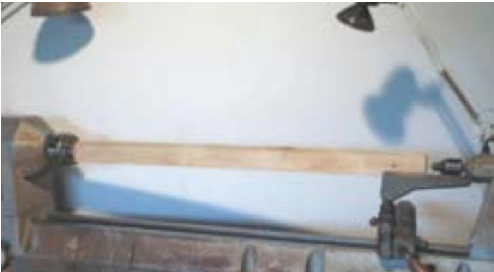
Figure 3. A length of wood mounted in a chuck.
