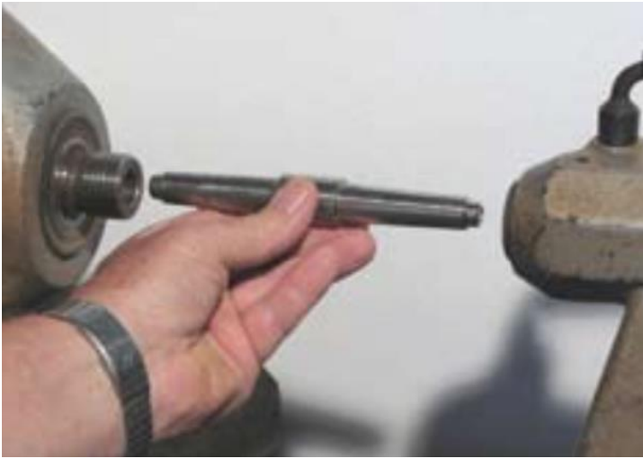
Figure 2. Using the Acruline System to check alignment.
