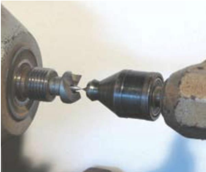
Figure 1. Using two centers to check alignment.
